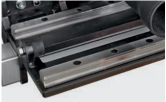
A rigid structure and linear guides with ball blocks guarantee excellent stability and machining precision over time.
